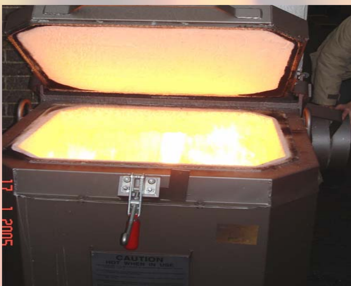
View of primary chamber during operation
